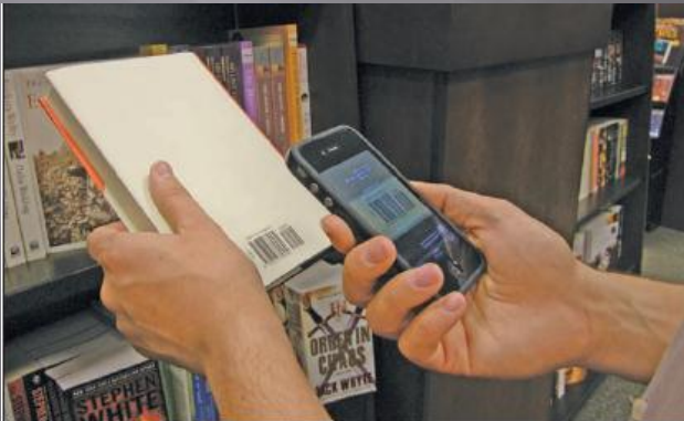
The RedLaser shopping comparison application for the iPhone takes a picture of a product's bar code and lists the prices for that item at various local retailers.
